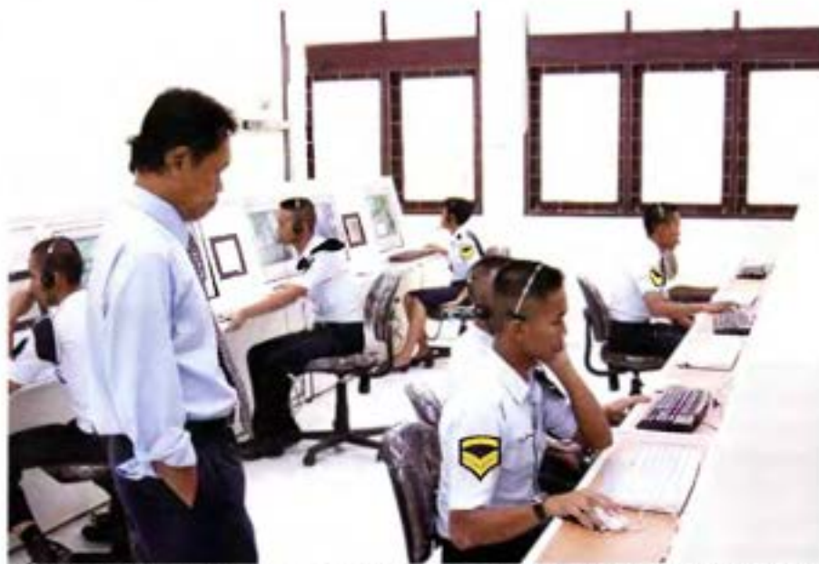
Modern training simulator complexes, such as that recently installed for the Indonesian Department of Civil Aviation, can accommodate over 60 separate training positions covering both radar and tower operations.
