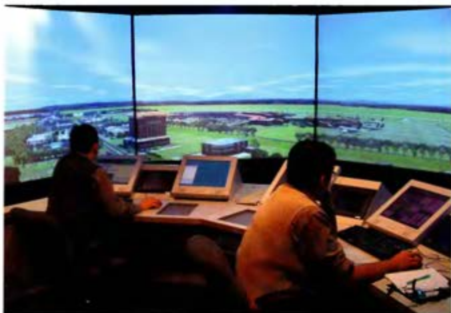
Students are shown in an office-sized 225-degree tower simulator designed for small rooms. The simulation in this example features Jakarta International/Soekarno-Hatta Airport.
