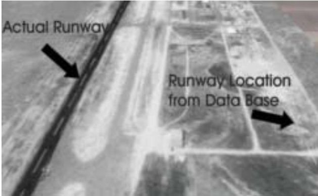
Figure 4. An error in database manipulation can cause a substantial offset in the designed approach from the actual runway, as evident in this example featuring Runway 26 at Moriarty, New Mexico.
