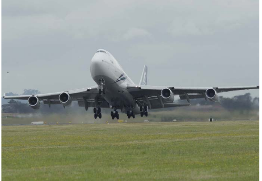
Air New Zealand's Boeing 747-400, powered by Rolls-Royce RB211 engines, takes off from Auckland international Airport last December. One of the four engines was run on a 50/50 mix of second-generation jatropha biofuel and Jet A1.
