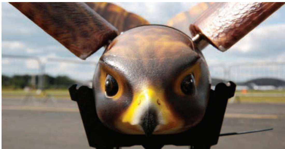
The "Robird," a drone which mimics the flight of a falcon, will be integrated into the Edmonton, Canada airport's wildlife management programme. Developed by Clear Flight Solutions and Aerium Analytics, Robird will help guide birds safely away from air traffic while discouraging nesting near airside operations and glide paths.
