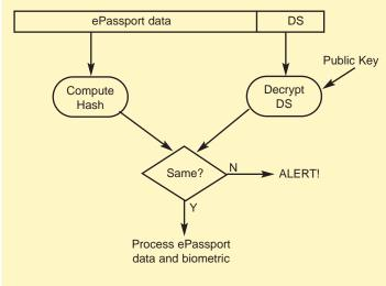
Figure 2 - Verifying the Digital Signature on an ePassport
