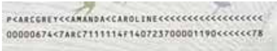
Figure 3. A sample of the OCR-B characters used in the passport's machine readable zone. As per ICAO Doc. 9303, II-2, machine readable information is contained in two lines of OCR-B text, each containing 44 characters.
