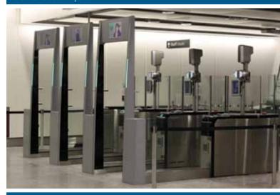
The Automated Border Control system at Heathrow Airport, Terminal 5.
