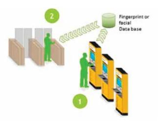
The Automated Border Control two-step process.
