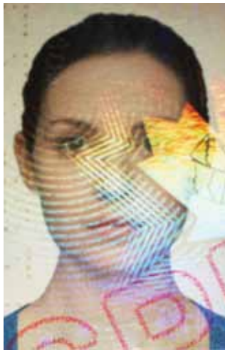
Security laminate contains a variable size text spiral, animation effects and an embossed effect in shape of map of Canada to protect bearer's photograph.
