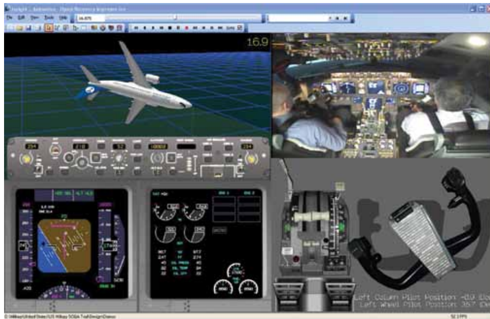
The online LOC-I training scenario for simulator instructors features an attempt to recover from a nose-low, high-bank upset condition in the Boeing 737 FFS.
