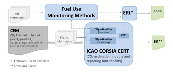
Figure 2: Architecture of CORSIA reporting system (2019 onward for compliance purposes)
