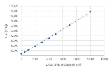
Figure 11: Illustration of generic aircraft CEM
