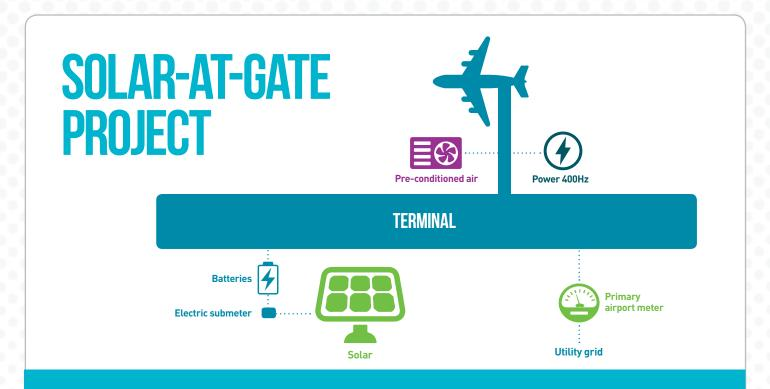
To power on-board systems and provide heating and cooling, most aircraft use their Auxiliary Power Unit (APU), typically located on the aircraft tail. The "Solar-at-Gate Project" is a two-step process to eliminate these emissions through a 100 per cent carbon-free solution:
