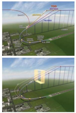
Figure 4 (top). Adjustment of the descent speed schedule can alter timing by two minutes or less when traffic conflicts require. Figure 5 depicts the use of a descent profile "window" for managing adjacent traffic streams.
