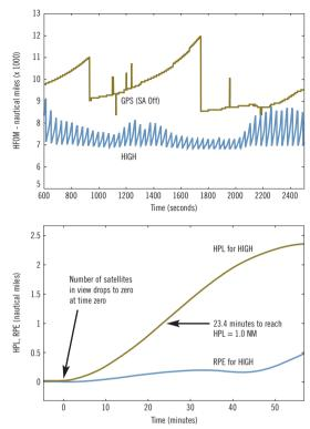
Figure 4 (top). Horizontal figure of merit (HFOM) for High Step II and GPS receiver. Figure 5. Integrity coasting demonstration illustrates HPL and RPE during simulated coasting conditions.
