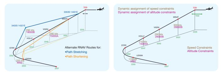
Figure 2 (left). With tailored arrivals in place, traffic conflicts are addressed by extending or shortening the distance flown and duration of descent by two minutes or more. Speed and altitude constraints (Figure 3) are also adjusted for the same purpose.
