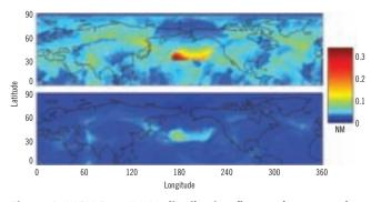
Figure 6. HIGH Step II HPL distribution (bottom) compared to HPL distribution from snapshot RAIM system.
