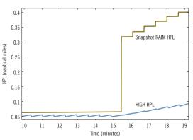
Figure 3. Simulation comparison of the horizontal position error in a RAIM hole
