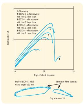
Figure 1. Changes in the maximum coefficient of lift and the critical angle of attack with different degrees of icing on the wing surface.
