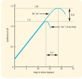
Figure 2. Results of wind-tunnel studies of the effects of very thin layers of ice on a full-scale Yak-40 wing with flaps extended 11 degrees.
