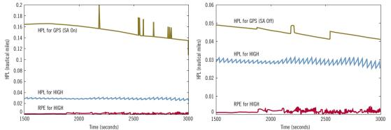
Figure 1 (left). Horizontal protection level (HPL) for the HIGH Step II navigation system and for a GPS receiver (SA-on) during flight test. Figure 2 (right). HPL for HIGH Step II system and GPS receiver (SA off).
