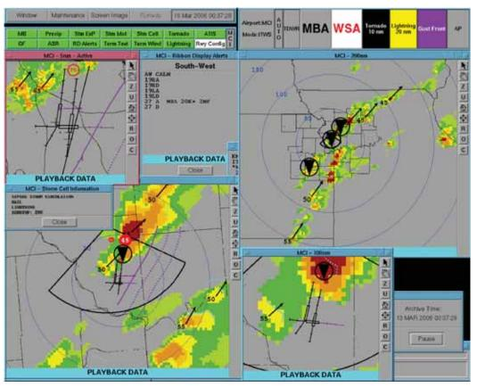
Example of ITWS display of severe weather containing microbursts, a gust front and tornados (Kansas City, 13 March 2006). ITWS features a prediction product that forewarns of a microburst
