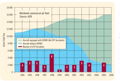
Mandated operation of EGPWS/TAWS has brought impressive results: to date, no aircraft equipped with this technology has suffered a CFIT accident
