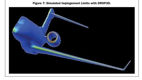
surface heat fluxes and shear stresses computed by the FENSAP module, the ICE3D module predicts the ice shape accreted on the entire aircraft's surface. Rather than assume empirical data for surface roughness, a new model analytically predicts the evolving surface roughness in space and time depending on whether it is metal and whether it is covered by a bead, a rivulet or a water film.
