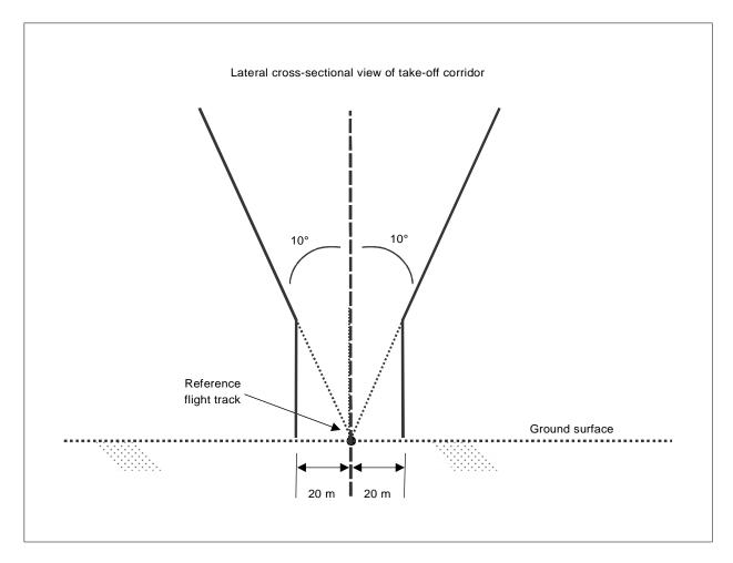
Figure 4-4. Lateral deviation tolerances for take-off
