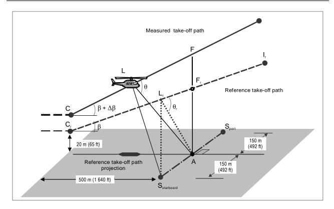
Figure 4-3 Comparison of measured and reference take-off profiles
