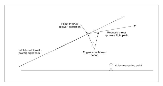
Figure 4-15. Take-off flight path over flyover measuring point with thrust (power) reduction
