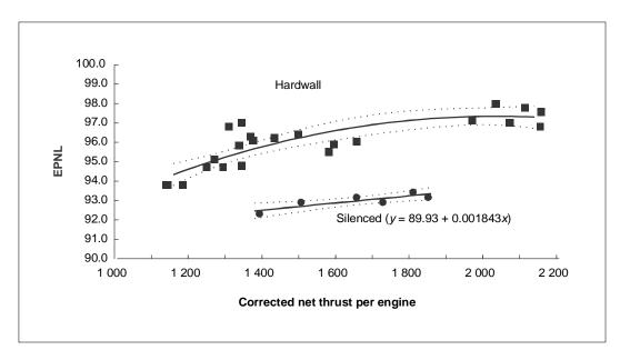
Figure 3-3. Regression curves for plots of EPNL against normalized thrust for hardwall and silenced conditions
