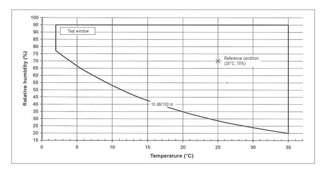
Figure 6-1. Appendix 4 temperature/relative humidity test window
