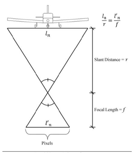
Figure 3.2.2.1 – Basic photo-scaling geometry
