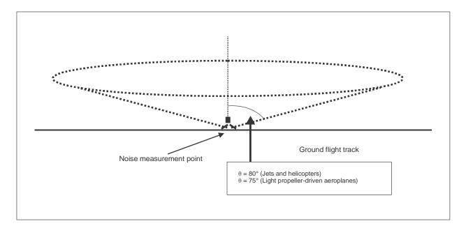
Figure 3-1. Obstruction-free cone defined from the base of the measurements microphone
