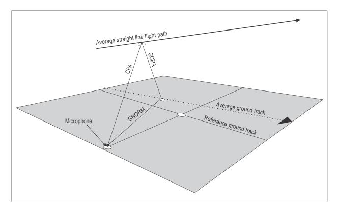
Figure 4-32. Basic CPA geometry
