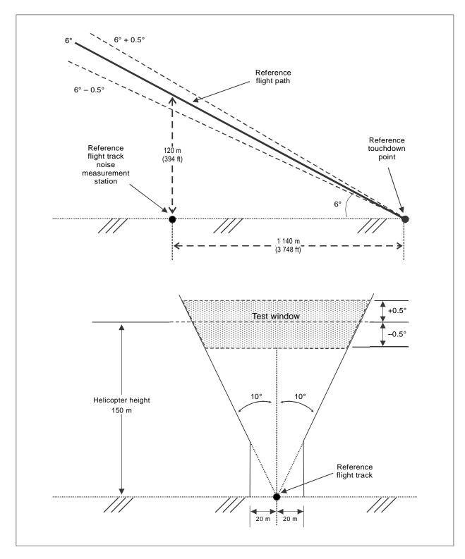
Figure 4-13. Flight boundaries for approach test condition
