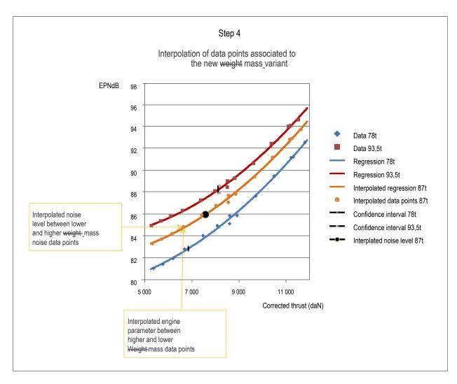
Figure 4-23 e). Calculation of confidence intervals for the interpolated masses
