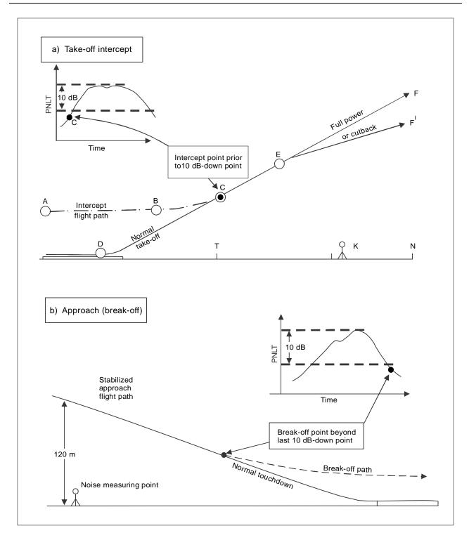
Figure 4-20. Flight path intercept procedures
