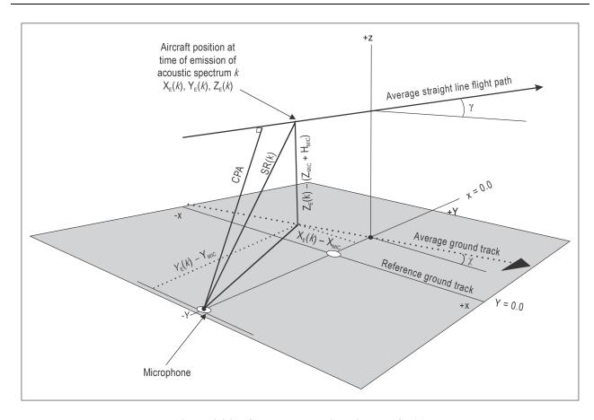
Figure 4-34. Sound propagation distance, SR(k)
