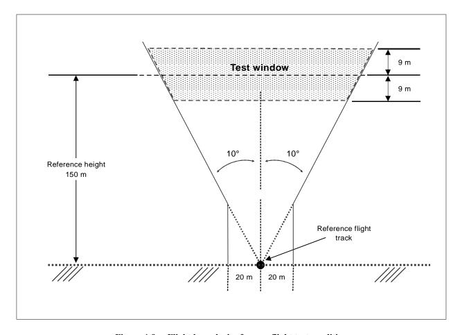
Figure 4-9. Flight boundaries for overflight test condition
