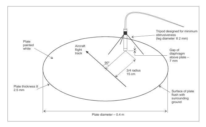
Figure 5-1. Configuration for one-half-inch inverted microphone
