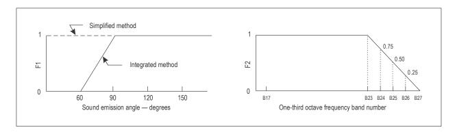
Figure 4-39. Criteria for jet source noise correction
