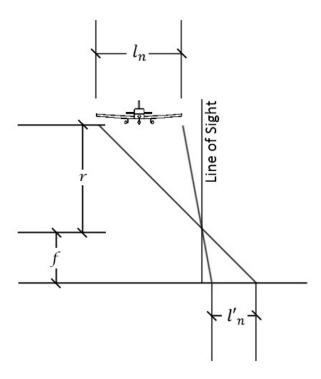
Figure 3.2.2.6 - Aircraft offset from overhead
