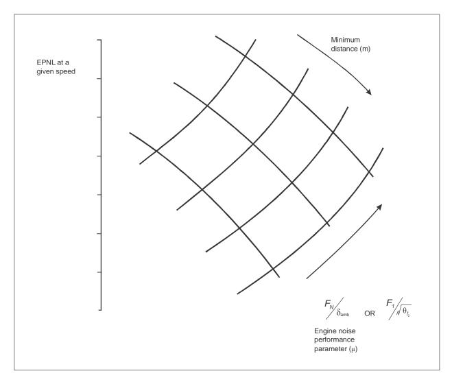
Figure 4-21. Form of noise-power-distance (NPD) plot for jet-powered aeroplanes
