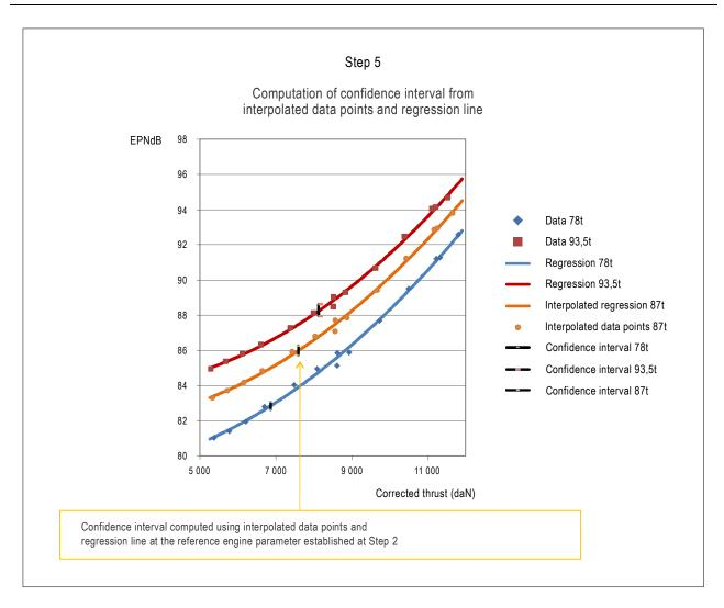
Figure 4-23 f). Calculation of confidence intervals for the interpolated masses
