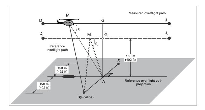
Figure 4-8. Comparison of measured and reference overflight profiles
