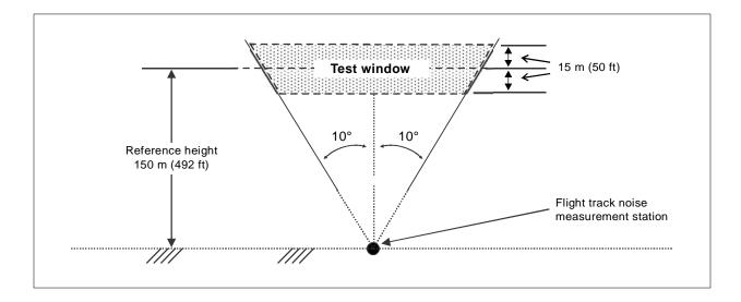
Figure 6-2. Flight boundaries for overflight test condition
