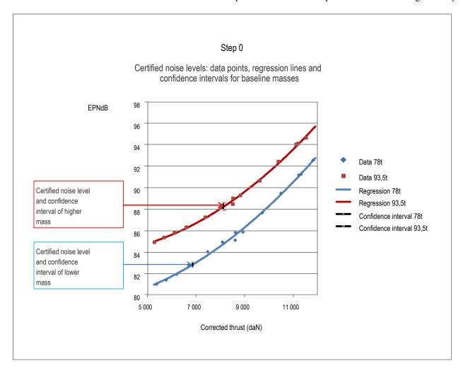
Figure 4-23 a). Calculation of confidence intervals for the interpolated masses
