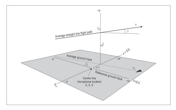
Figure 4-30. Single-point flight path descriptors
