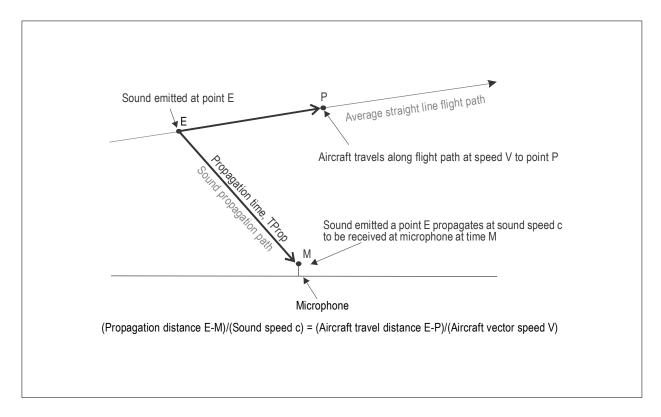
Figure 4-31. Aircraft position at time of sound emission
