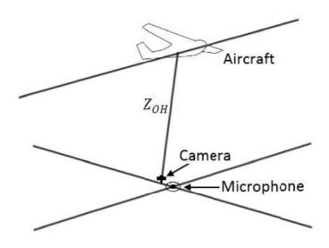
Figure 3.2.2.2 - Notional geometry for certification noise testing
