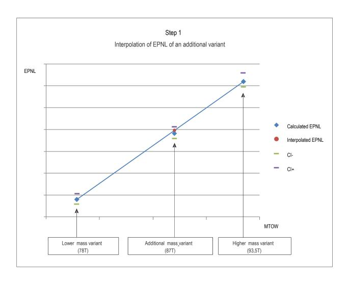
Figure 4-23 b). Calculation of confidence intervals for the interpolated masses
