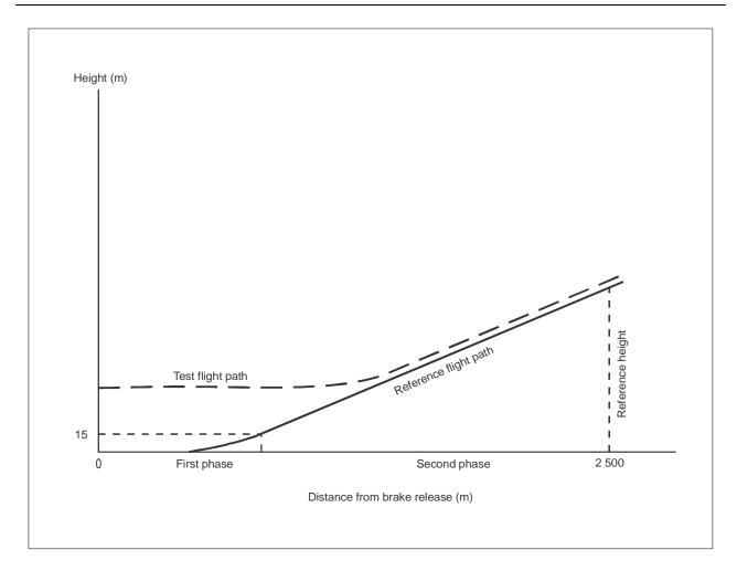
Figure 5-2. Typical test and reference profiles
