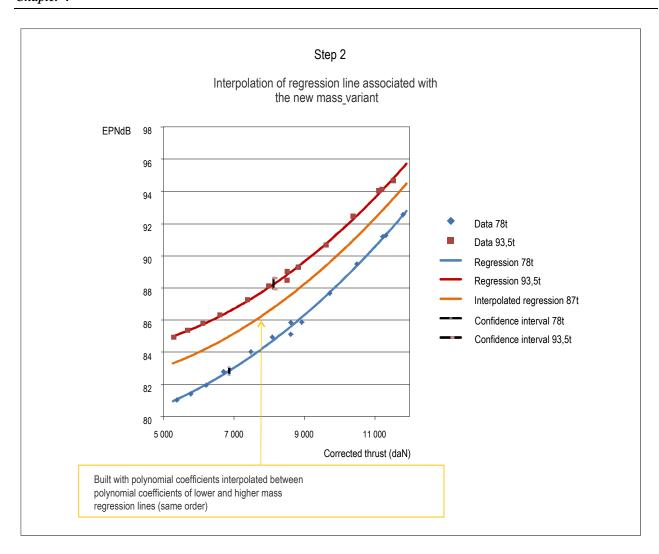
Figure 4-23 c). Calculation of confidence intervals for the interpolated masses
