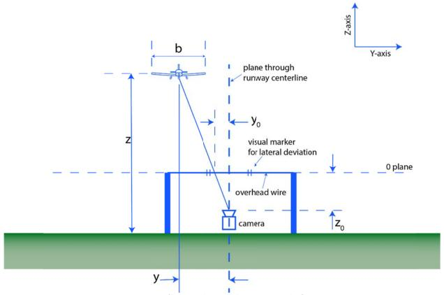
Figure 3.2.2.3 - Profile view schematic illustrating visual reference wire
