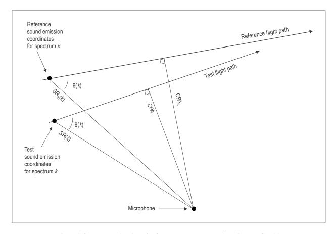
Figure 4-37. Determination of reference sound propagation distance, SR<sub>R</sub>(k)
