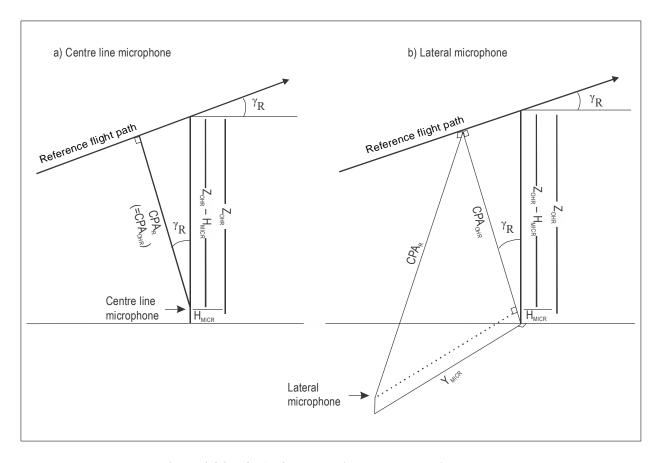
Figure 4-36. CPA<sub>R</sub> for centre line and lateral microphones
