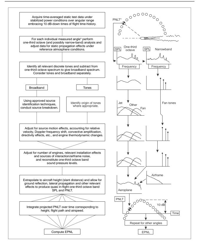
Figure 4-26. Example procedure for projection of static engine data to aeroplane flight conditions
