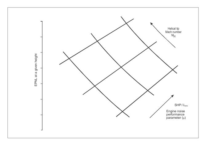
Figure 4-27. Form of noise-power-distance (NPD) plot for heavy propeller-driven aeroplanes
