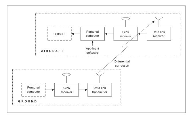
Figure 3-2. DGNSS TSPI system basic architecture
