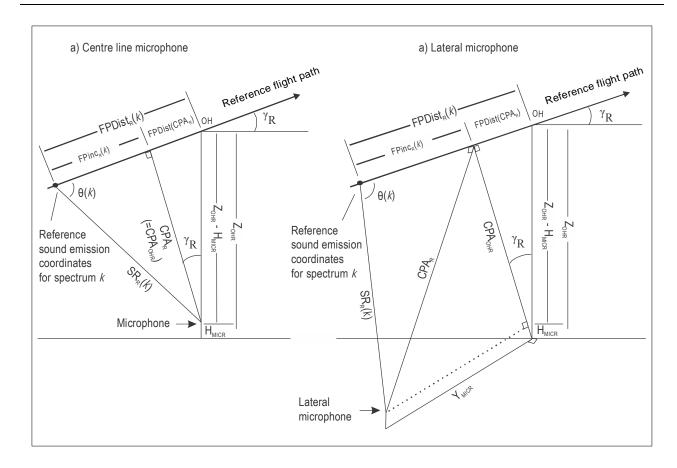
Figure 4-38. FPDist concept for centre line and lateral microphones
