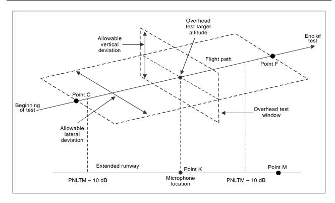
Figure 4-17. Take-off flight path tolerances
