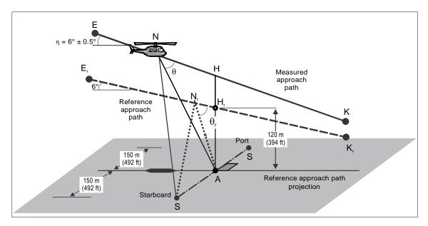
Figure 4-12. Comparison of measured and reference approach profiles
