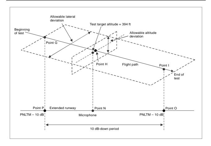
Figure 4-19. Approach flight path tolerances
