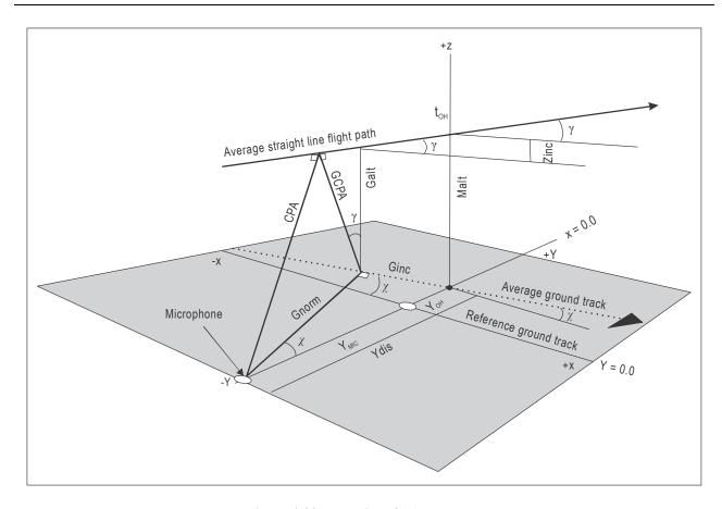
Figure 4-33. Detailed CPA geometry
