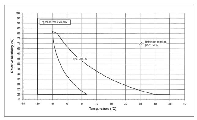
Figure 6-3. Optional Appendix 2 temperature/relative humidity test window
