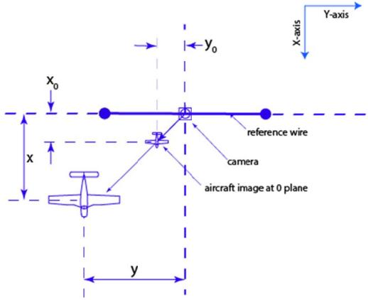
Figure 3.2.2.4 Plan view schematic illustrating visual reference wire
