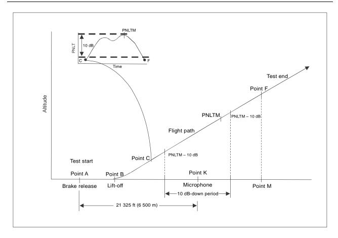
Figure 4-16. Normal full thrust (power) take-of
