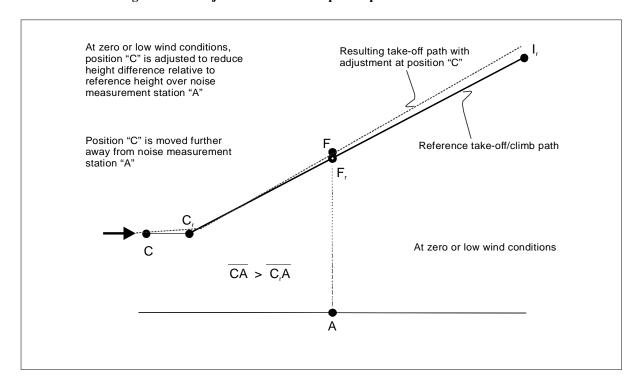
Figure 4-6. Adjustment of take-off profile position "C" for zero or low wind
