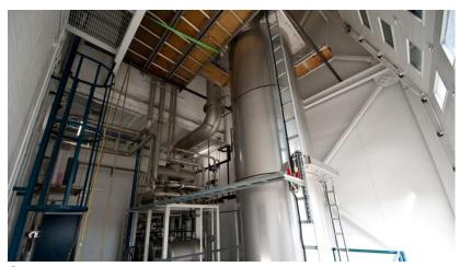
Step 3 Distillation tower Glycol concentration is increased by distillation to 99.5%.
