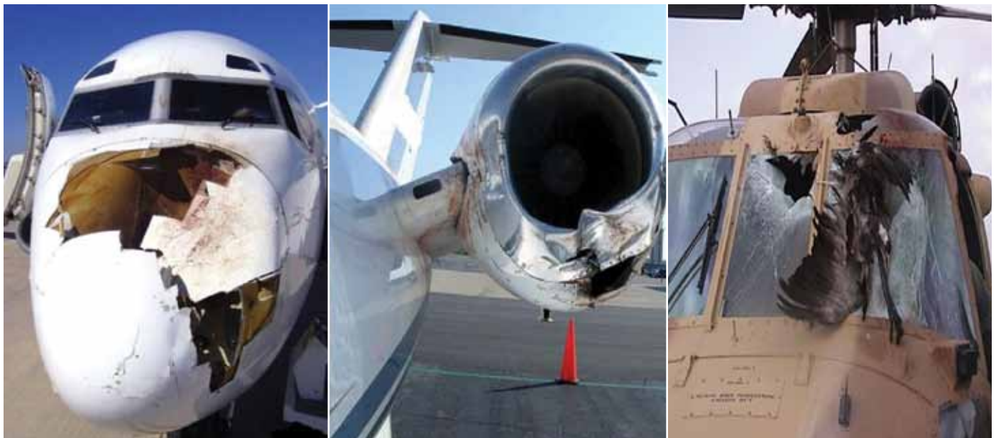
Some examples of the damage that can be caused to aircraft and engines as the result of bird strikes. A total of 6996 bird strikes were reported by 18 States in the Asia/Pacific Region between 1996–2006.
